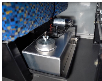
5-Gallon Reservoir mounted under seat
